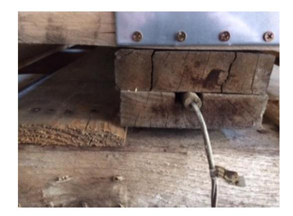
In this example, the adjoining deck boards are thicker than the stringer the thermocouple is placed in. A surrogate block that is as thick or thicker than the combined thickness of the adjoining deck boards should be employed to position the thermocouple.
