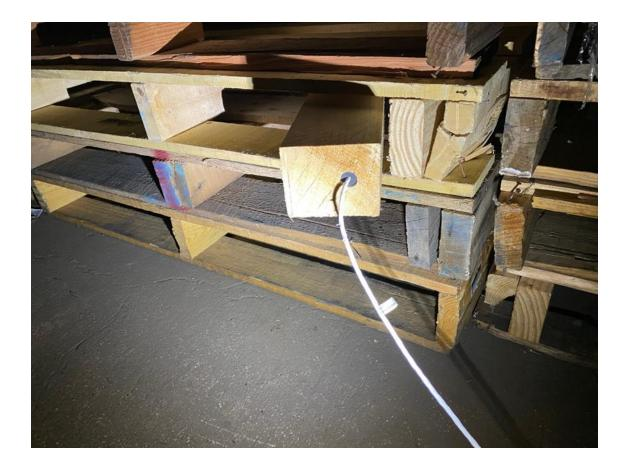
The surrogate block used for the thermocouple is not properly drilled in the center of the block. Offset holes in surrogate blocks are not allowed.
