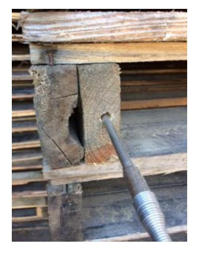
The thermocouple in this example is sandwiched between two adjoining pieces of wood. This is nonconforming no matter how tight the joint is. A surrogate block should have been used for the proper placement of the thermocouple.
