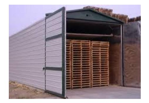
Heat chambers manufactured and assembled by an approved original equipment manufacturer (OEM) typically do not require a verification study by an agency when they operate at minimum core temperatures of 140°F.
