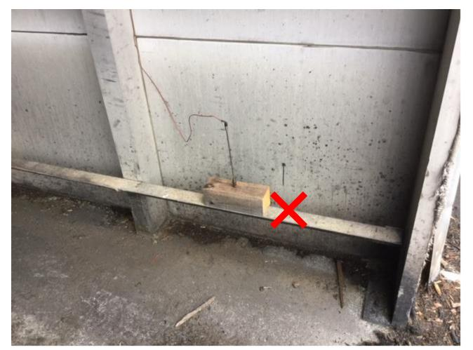
When companion stringers are used in the repair of WPM, the combined thickness of the two pieces must be used to determine the thickest wood in the chamber. This thermocouple was placed in a single stringer which would not be considered the thickest piece of wood.
