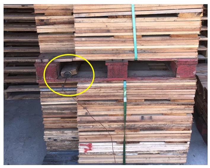
The holes in these surrogate blocks were drilled so big the thinner walls would not accurately verify the proper heat treating of the thickest solid piece of WPM.
