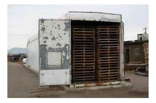
Heat chambers created from insulated trailers or other structures that are customized with equipment to provide heat and record core temperatures, require a verification study. This study verifies the customized chamber meets ISPM 15 requirements along with determining thermocouple location, and ensuring all equipment is properly operating.
