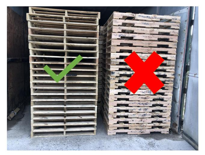
Pallets should be arranged so that stringers are aligned with or parallel to the air flow. Pallets should not be placed in the heat chamber where they greatly restrict airflow.
