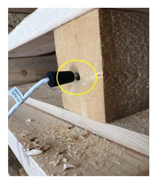
The surrogate block shown is not in the coldest area of the heat chamber. The metal it sits on could also heat the block faster than the associated WPM in the chamber.
