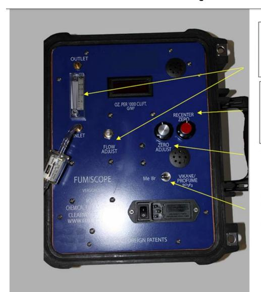
FLOW ADJUST indicates the amount of gas sample being drawn through the unit. The flow meter may need to be adjusted after sample lines are attached and/or disconnected. The flow rate must always read 1.0.
