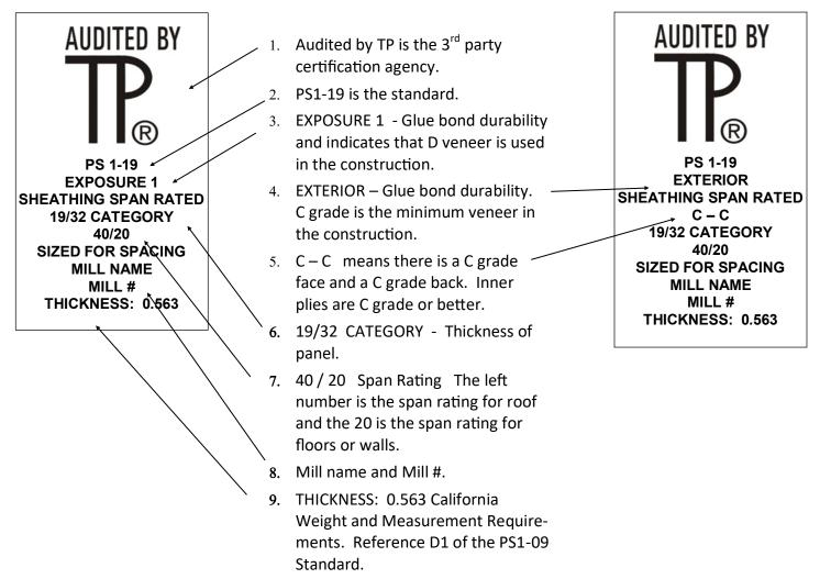
Sheathing Span Rated Panels, CD Sheathing Span Rated, and CC Sheathing Span Rated are interchangeable with other certification agencies. Reference the standard for sheathing product requirement and not the certification agency. Rated Sheathing (APA), Sheathing Span (TECO) and Sheathing Span Rated (TP).
