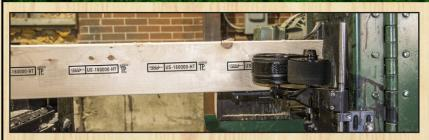
For higher volume applications, automatic marking provides continuous imprints without the need for constant attention.
