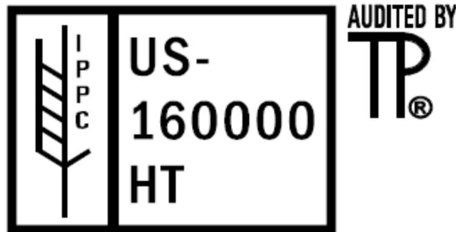
Anytime a pallet is repaired, it puts into question the conformance of the material it was repaired with. The American Lumber Standard Committee (ALSC) has stated that any pallet that appears to have been repaired or altered needs to have the old marks obliterated (made completely unreadable) before it can leave the facility. Retreatment must occur before a new IPPC mark can be applied.
