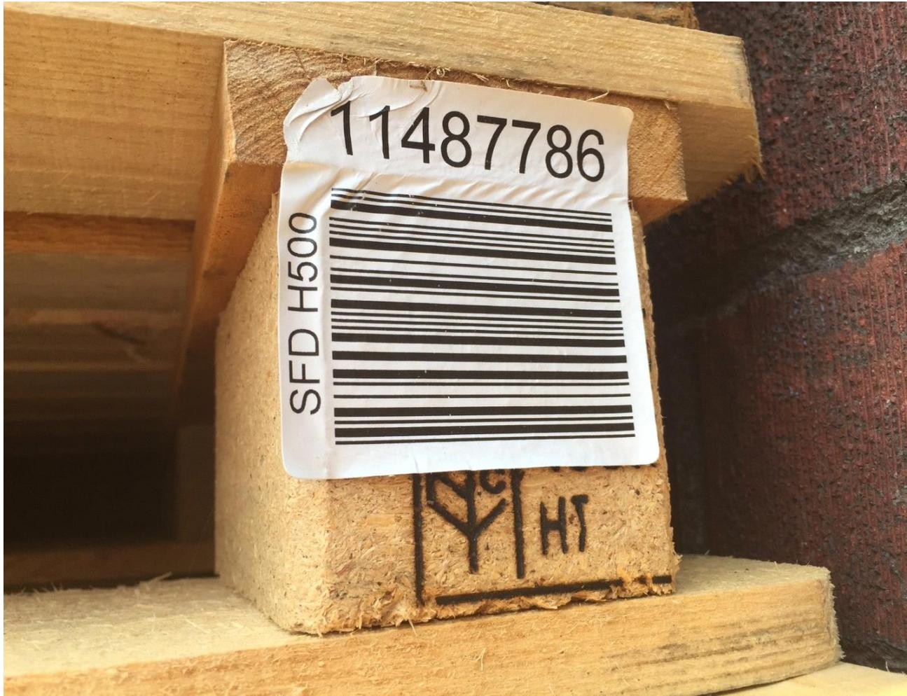
A sticker covering a mark is NOT obliterating the mark. The stickers should be removed and the mark covered with paint.
