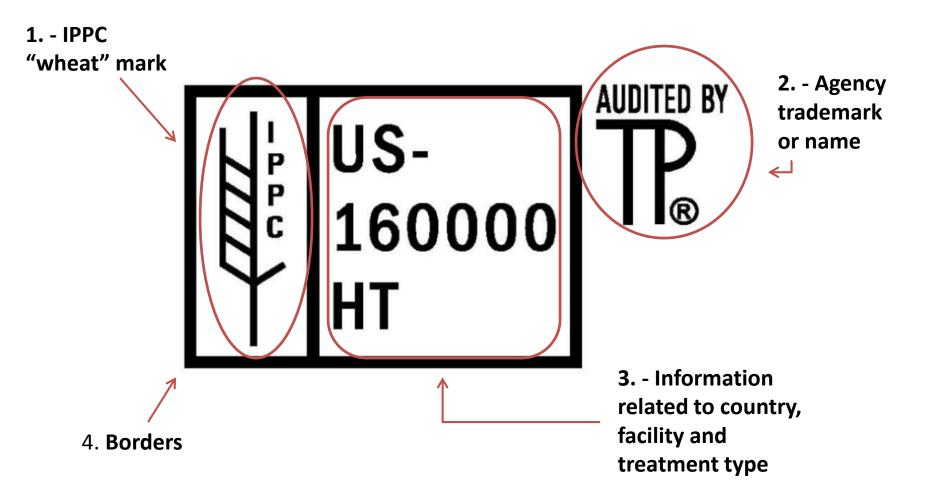
For obliteration to meet requirements all 4 parts of the mark must be covered with a permanent substance (i.e. paint) that renders it undiscernible.
