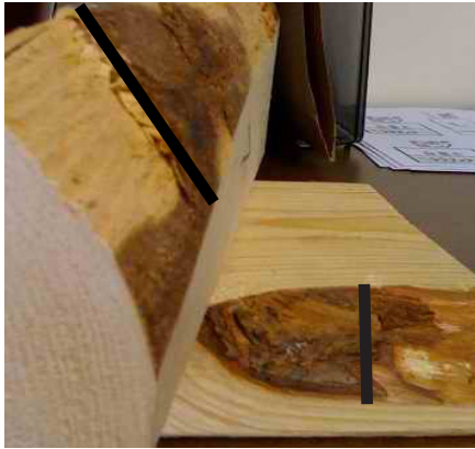
Fig. 1: Measure bark across the contoured surface at its greatest width
