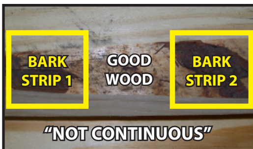
Each strip of bark is completely surrounded by "good wood" (or non-bark). Individual strips should be evaluated separately.
